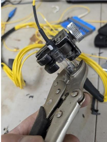
and made a circular cut around the splice tube which allowed the fibers to extend out thus removing the microbends of the worst offending splices. And then lastly, Aristo Networks secured the previously opened splice tube by re-applying heat shrink over the splice tube. While not every splice could be fixed using this method, nearly all splices could be brought back into spec using the above method.
